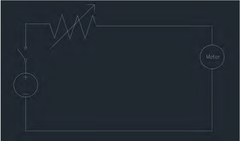
Figure 8: Wiring diagram for drop device
