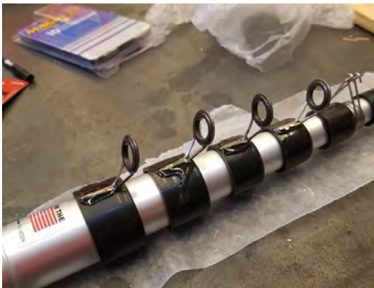
Figure 10: Original Cable Guides
