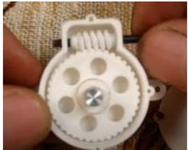
3D Printed Worm Gearbox from YouTube
