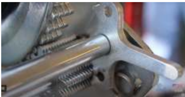
Reversible Ratchets on Pulling Winches from Dutton-Lainson
