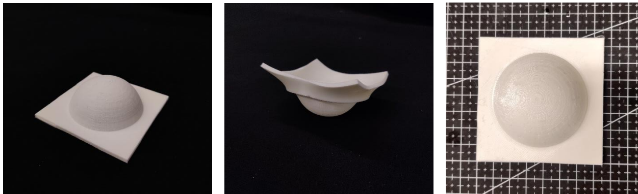
Figure 2 – Scale down version of silicone rubber casting of single dome structure. Overall structure will be roughly 20cm in length and breadth with a dome height around 7.5cm. From left to right: Single unit dome in its as-cast state, inverted state after interaction and top view for scale (1 square:1cm)
